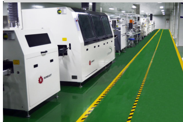
PCB Coating Line
